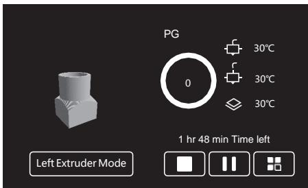
5. The printer starts to heat up and will start printing after heating completed.
