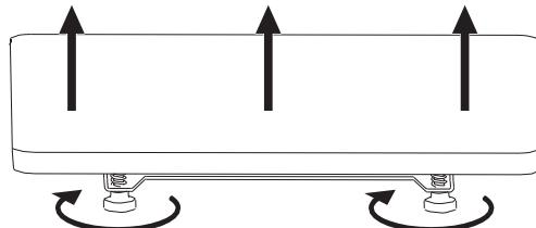
**Rotate the nut clockwise**
