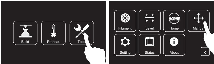
11. Plug power cable into the input on the back and turn on the power switch. Tap[Tools],[Manual].
