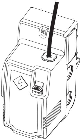
6. Insert filament guidetube into filament intake to fix.
