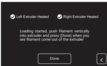
4. Once heated, filament will be drawn through the extruder. Continue extruding until the extruder provides a steady flow of filament. Tap [Done], go back. Tap leftwards arrow to go back to the home screen.
