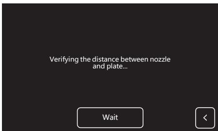
3. After leveling extruder confirmed,extruder will move to the first point to verify the distance between nozzle and build plate. If verify completed, extruder will move to the second point to verify the distance.
