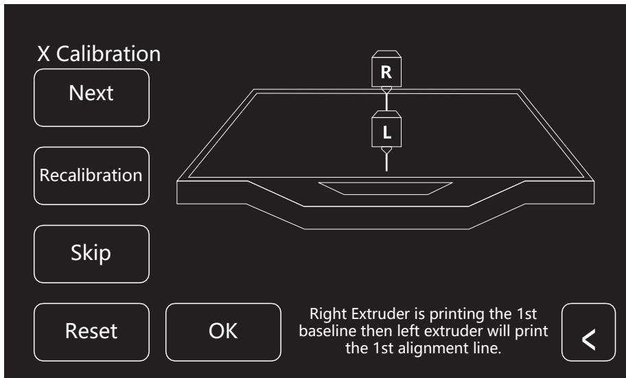
1. Tap [X-axis calibration] and wait for extruders heating up. After heating up till target temperature, 2 lines will be printed in sequence. Check if the 2 lines are aligned after printing. Meanwhile, the pop-up window will appear.
