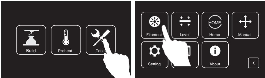
1. Tap[Tools], [Filament] to enter the filament interface.
