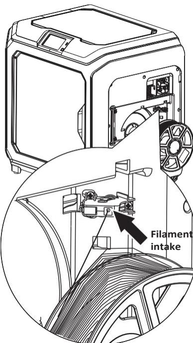
2. Insert the filament into filament intake.
