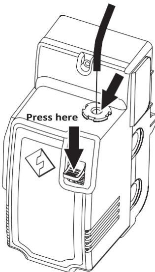
5. Press the spring presser, put filament vertically into the left filament intake to the bottom.
