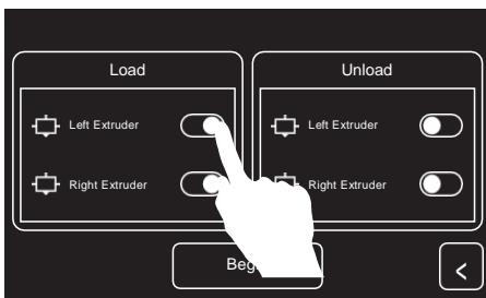
2. Flip the switch after corresponding extruder to load corresponding extruder.
