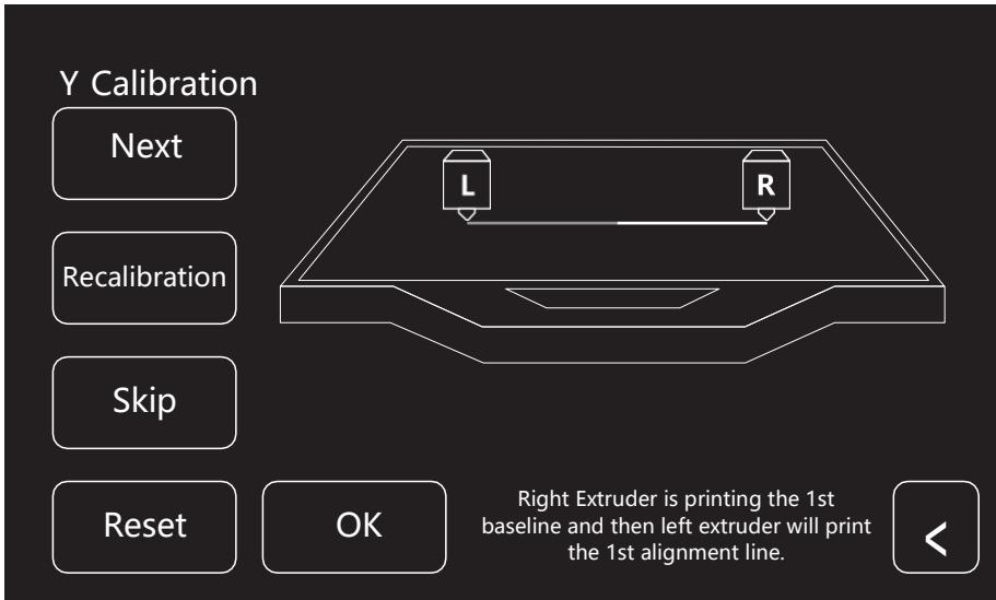
1. Tap [Y-axis calibration] and wait for extruders heating up. After heating up till target temperature, 2 lines will be printed in sequence. Check if the 2 lines are aligned after printing. Meanwhile, the pop-up window will appear.
