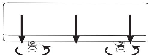
**Rotate the nut anticlockwise**
