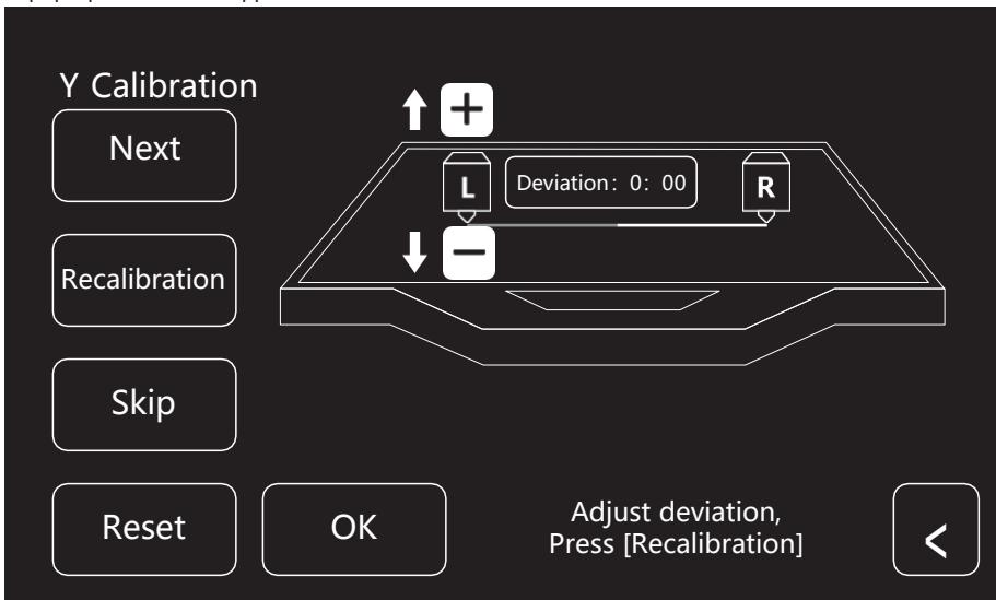
2. If the 2 lines are totally aligned, Tap [Yes], Y-axis calibration is done. If the 2 lines are not totally aligned, Tap [No]. Adjust position of extruders according to actual situation. After that, clean the filament on build plate and Tap [Recalibration]. Repeat step 2 till the 2 lines are totally aligned.
