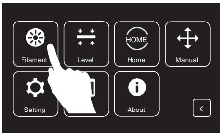
1. Tap[Tools], [Filament] to enter the filament interface.
