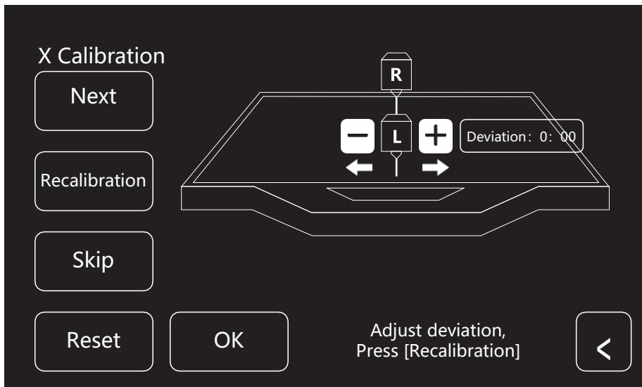
2. If the 2 lines are totally aligned, Tap [Yes], X-axis calibration is done. If the 2 lines are not totally aligned, Tap [No]. Adjust position of extruders according to actual situation. After that, clean the filament on build plate and Tap [Recalibration]. Repeat step 2 till the 2 lines are totally aligned.
