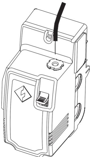
4. Insert filament into filament intake continuously until filament goes through filament guidetube.
